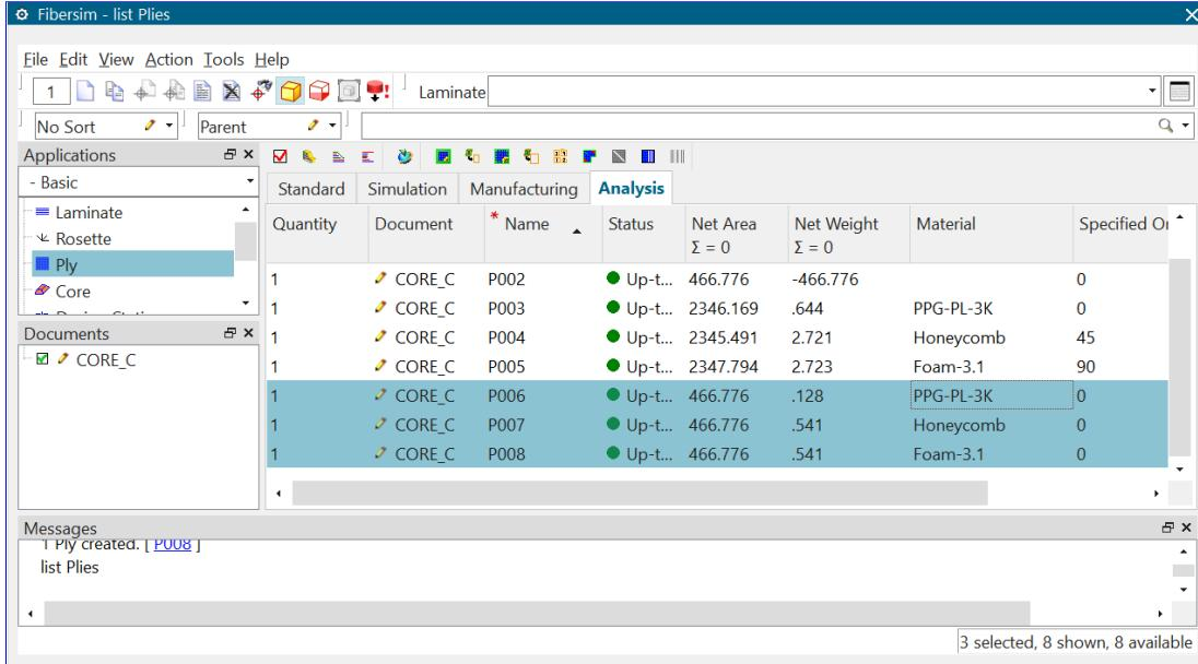
6) Make three plies with the materials mentioned above in the Inner Region in 3 different directions (**ppg-pl-3k = 0, honeycomb = 45, foam-3.1 = 90**) and show their difference in the figure.
